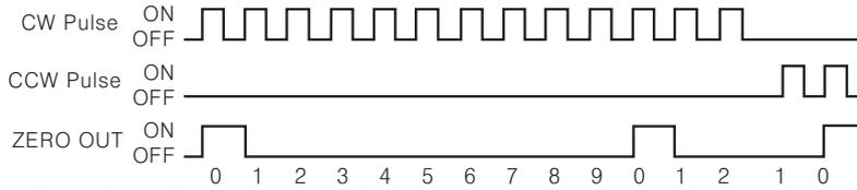
※The signal is output to indicate when the motor excitation status is in the initial stage. / Used to check the rotation position of motor's axis
