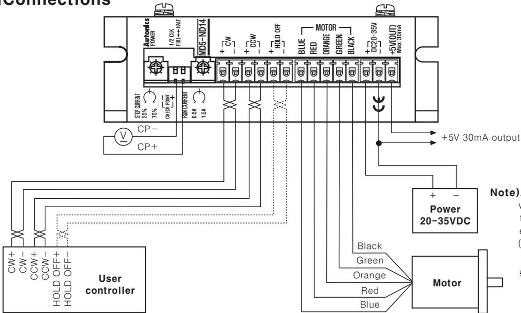
Note) Add external resistance when power for pulse from the external of the unit exceeds +5V. (Input current: 10 to 20mA)
