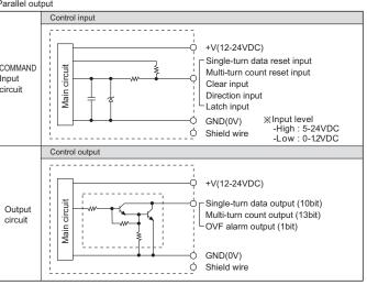
Output of each bit is the same circuit XOverload or short may cause circuit break
