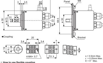
How to use flexible coupling When mounting the coupling to encoder shaft, if there is big eccentricity or bend between rotating encoder shaft and mate shaft, it may cause encoder and coupling's life cycle to shorten.
