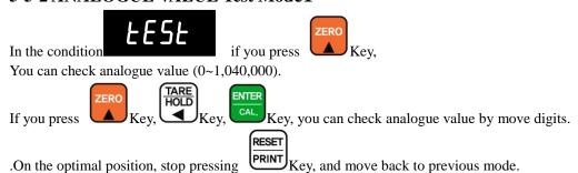
**\*\*** If the analogue value is unstable, or there is no change although pressing or loading some force on/in weighing part, please check load cell, load cell cable, connector, A/D board.
