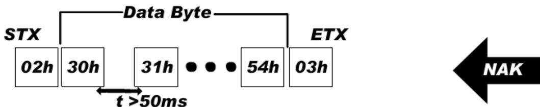
※Although wrong value is transmitted, the communication format is matched, then ACK is transmitted.
