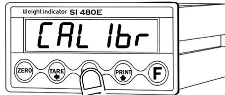
Under "SETUP" displays then Press
