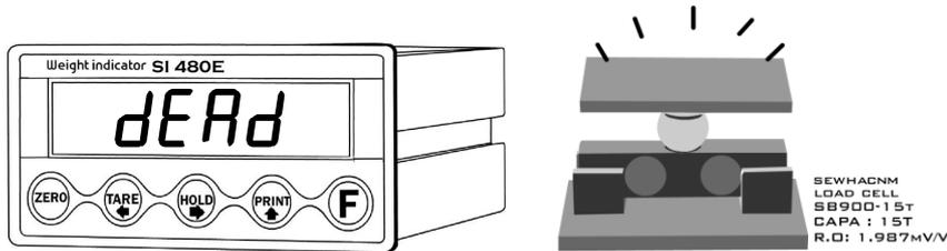
"dEAd" is displayed. Please press **F** key with empty scale. Then the indicator starts to measure and find optimal "Dead weight value of Scale" automatically.
