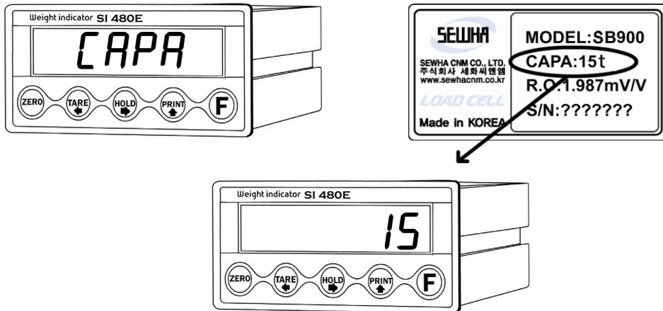
After "CAPA" displayed, Check Max. Capacity of Load cell.
