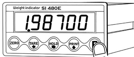
After "CAPA" displayed, Check Max. Capacity of Load cell.
