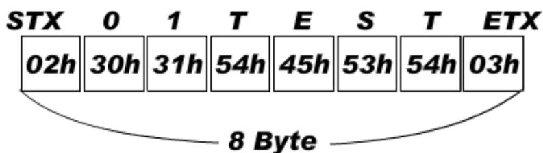
※ If you send "Testing protocol" from PC to Indicator, at the normal operation Display will blink.
