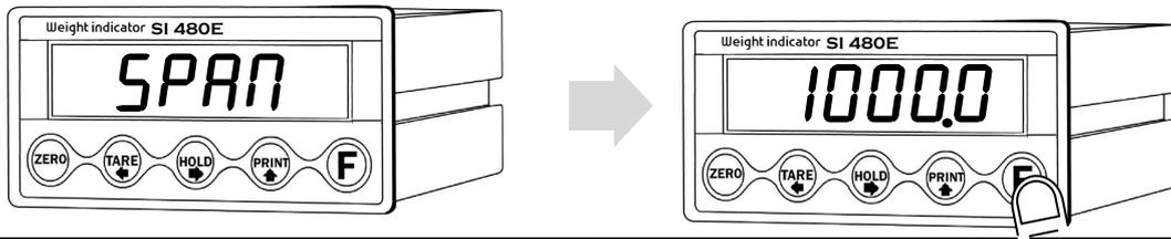
If "SPAN" is displayed, input "Test Weight" capacity and press
