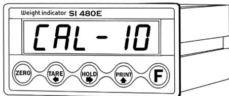
Calculate Span value during 10 ~20 secs, automatically.
