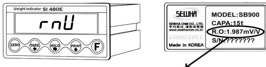
Input the output value load cell Following fixed decimal point.
