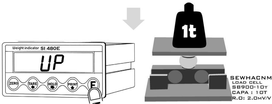
If "UP" is displayed, please load "Test Weight" on the scale part and press
