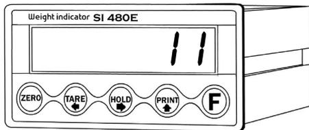
Under this mode, you can test Key input and Digital Key input test
