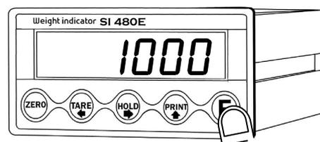
After displaying "CAPA", input max capacity with keys & Press
