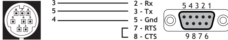
Motion Coordinator to 'AT' style PC with 9pin serial connector
