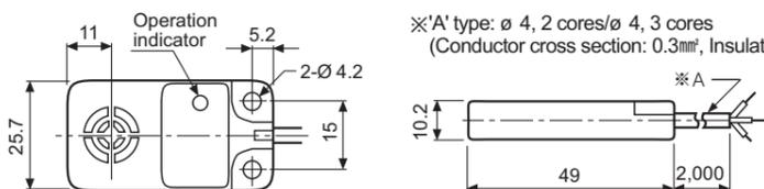
※'A' type: ø 4, 2 cores/ø 4, 3 cores
